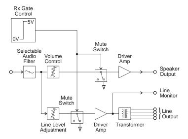
Figure 2.3 T835 Audio Processor Block Diagram
