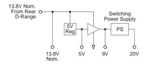
Figure 2.4 T835 Power Supply And Regulator Block Diagram
